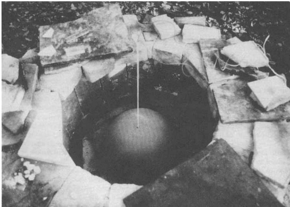
Figure 1. Kiln within the opened non-magnetic furnace. White rod: a thermocouple leading into the centre of the kiln.
